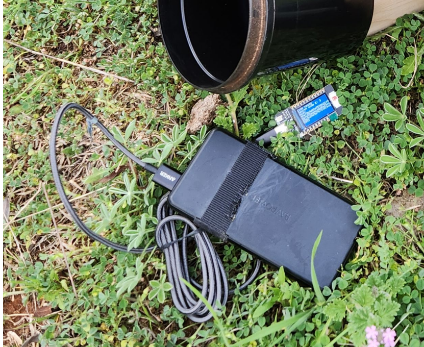
Figure 6b: A Lilygo T-Display board, running the sensor module software, connected to a 10,000 mAh battery and placed next to a bucket stand.
