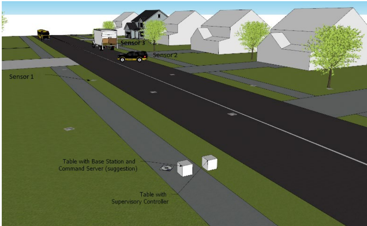
Figure 5b: An example of a view of the test area from the recording camera. Note that the UAV must stay in view for its entire flight. Multiple cameras may be used as necessary.
